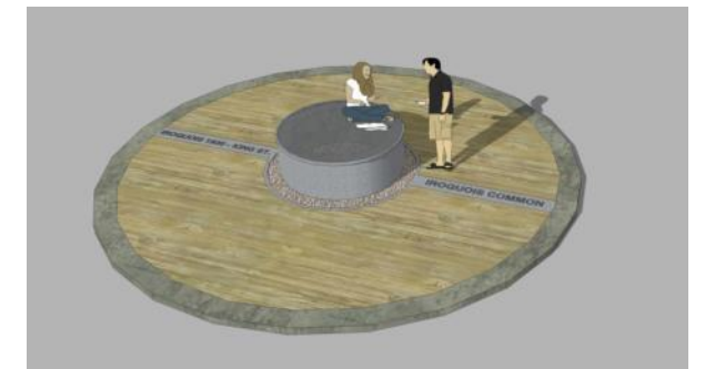
During regular days (without scheduled BBQ activities), a lockable metal lid will prevent visitors from using. With the metal cover in place, it also can be used as a bench or table.
