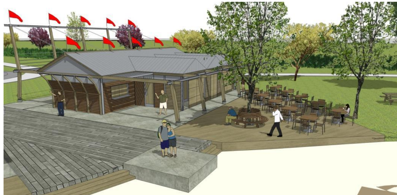
Image showing, an alternate Enhanced Beach Pavilion design. This option portrays a series of gable roof elements at south building addition, representing the nautical architecture of the typical boathouse (at Iroquois Marina area).
