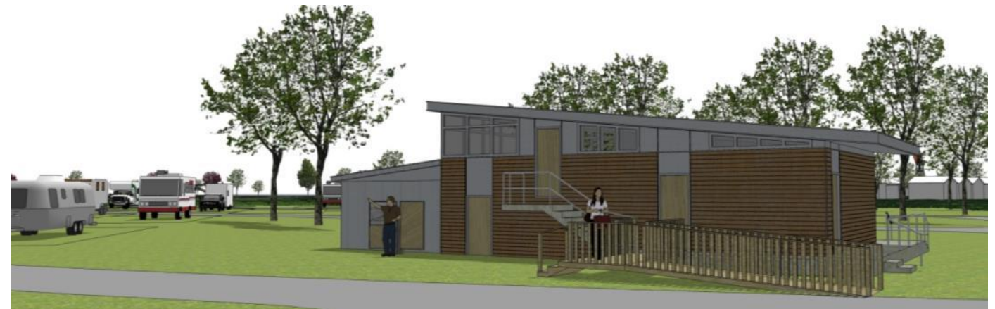
Fig. 40 - The existing campground administration building remains in place to save costs, but is enhanced with an inexpensive re-cladding to harmonize with the family of new interventions and their design materials.
