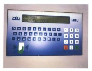
3. The GIR Controller will now ask for the Vehicle Badge. Hold the grey key fob between arrows on bottom left of controller.
