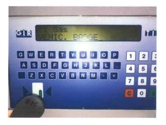
4. The GIR Controller will ask for the vehicle kilometers or hours. Please enter the proper kilometers/hours using the keypad and press the **E** to proceed.
