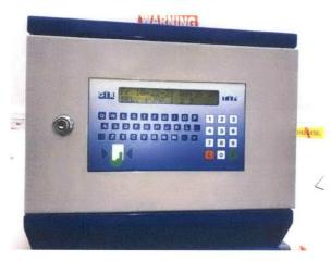
2. The GIR Controller will now ask for the Driver Code. Enter in your code by using keypad and press **E** to proceed.
